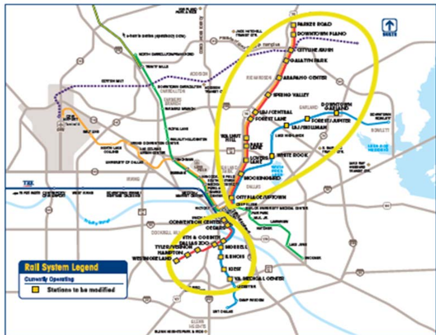
Along the Red and Blue lines, 28 light rail stations – which lie outside of Downtown Dallas and were built before 2004 – need to be lengthened and/or modified to accommodate three-car trains.
