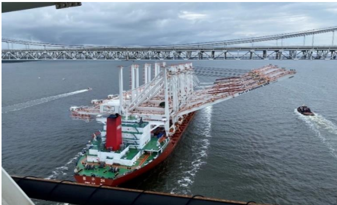
Four supersized Neo-Panamax cranes being delivered to support operations of a second 50-foot berth for Seagirt Marine Terminal at the Port of Baltimore.
