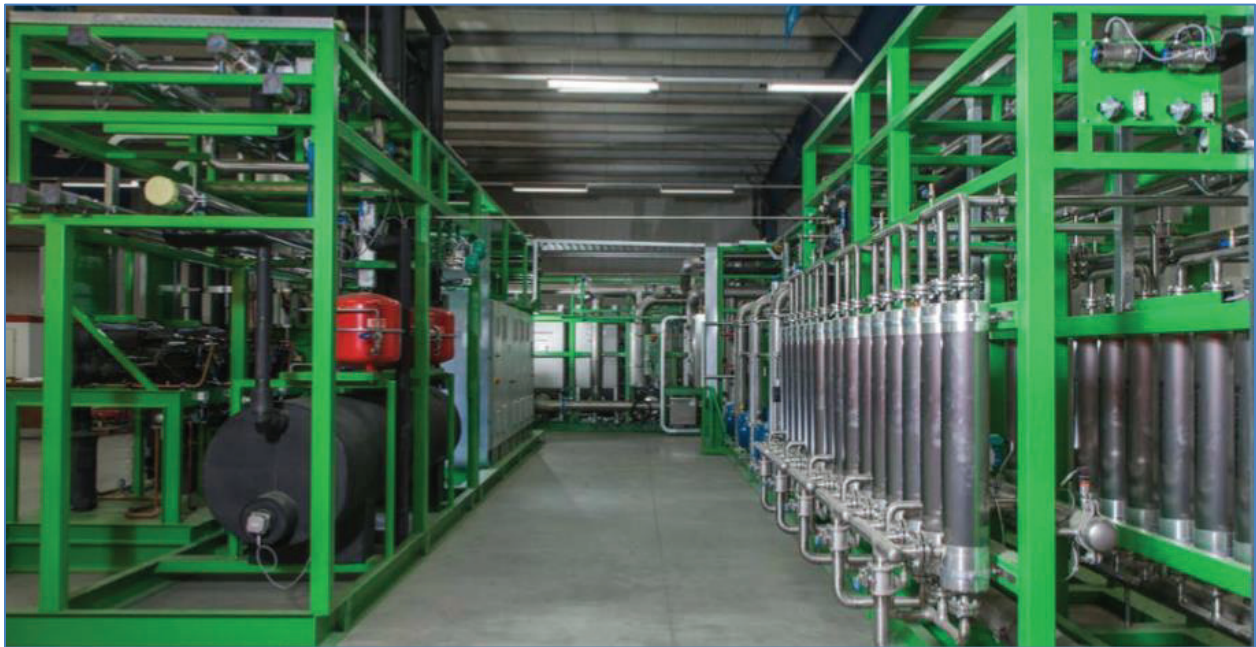
Figure 2-12 Biogas Upgrading System
