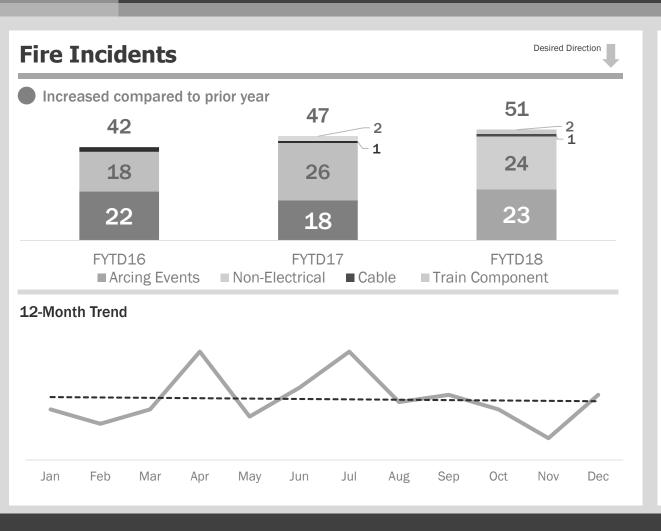
Increase in fire incidents driven by high rainfall in July, which led to a spike in arcing insulators; no arcing insulators in November or December
